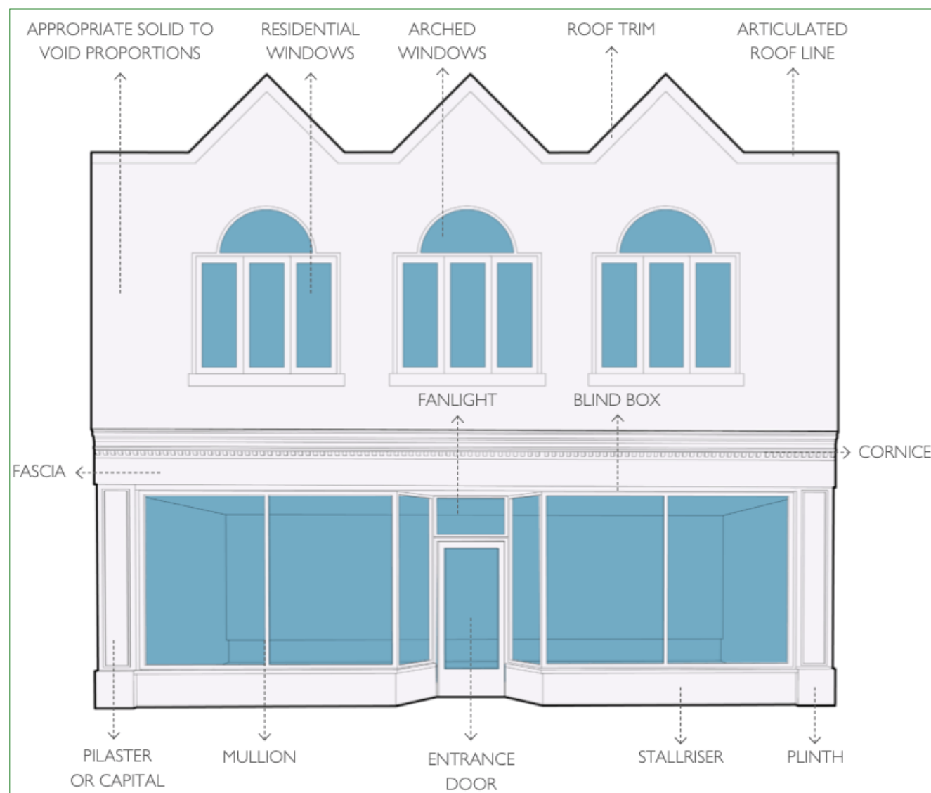
Figure 44: The key features and design principles of a traditional shopfront
